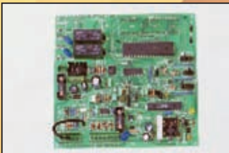
Description: Electronic Controller for Nuova Elettra LS3 Battery Charger
