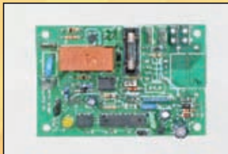
Description: Electronic Controller for Nuova Elettra RPE Battery Charger
