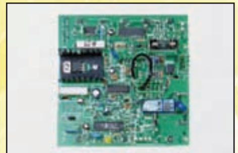
Description: Electronic Controller for Nuova Elettra RTM Battery Charger
