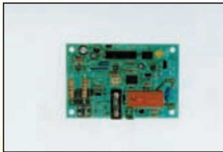
Description: Electronic Controller Nuova Elettra RPE Charger (State Voltage)
